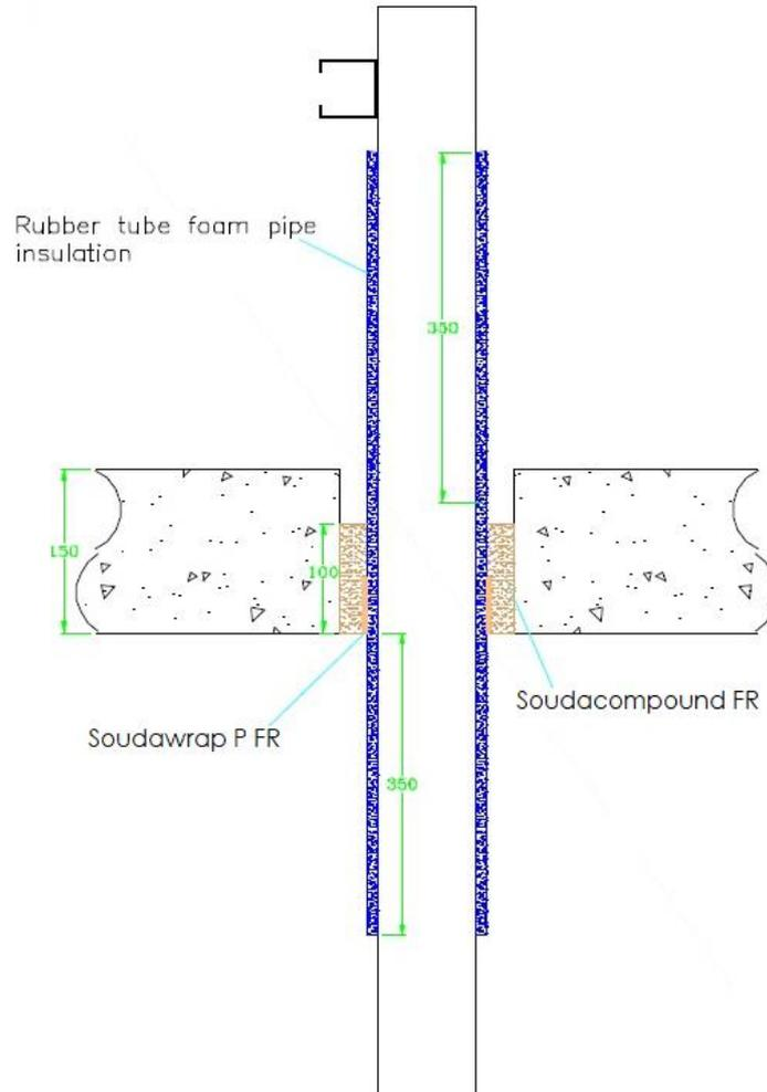
**A.2.5.1 Single side penetration seal with pipes**
