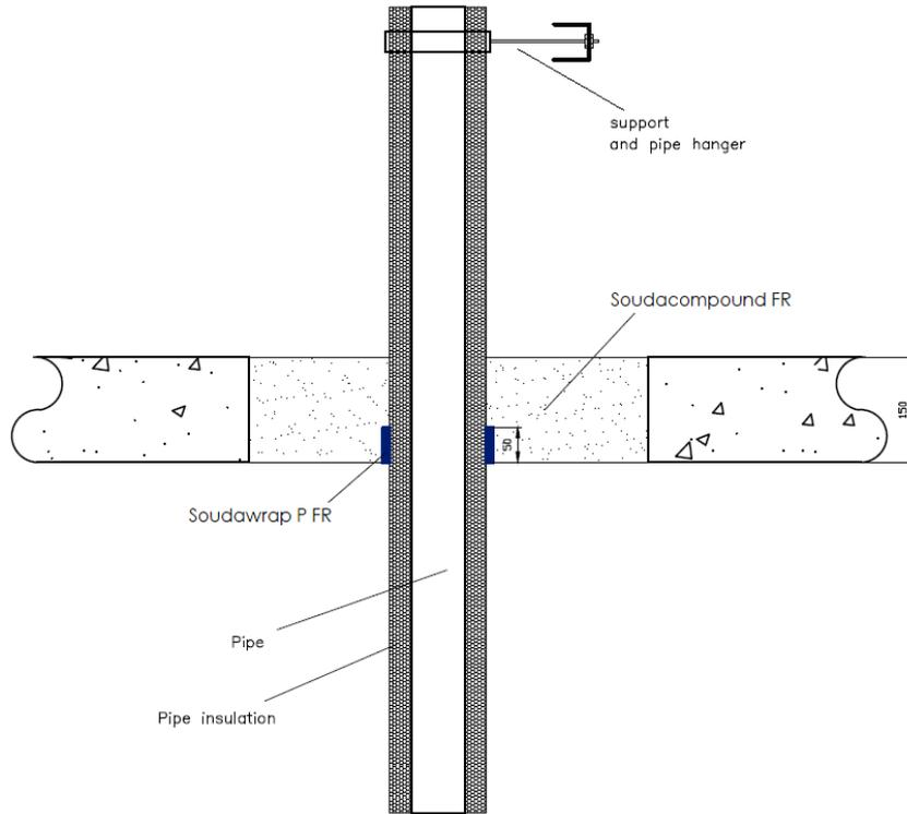
**A.4.1.1 Single side penetration seal with pipes**
