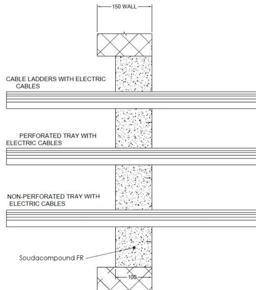
**A.1.4.1 Single side penetration seal with cables**
