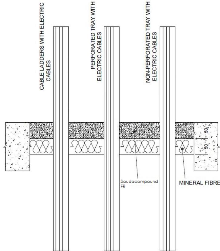
**A.2.1.1 Single side penetration seal with cables**
