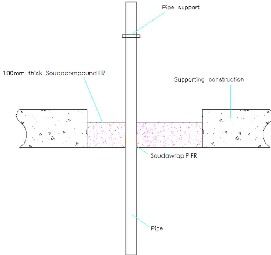
**A.2.10.1 Single side penetration seal with pipes**
