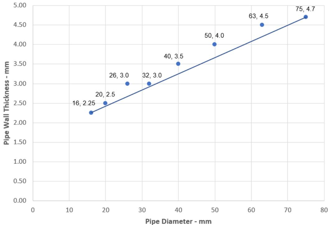
**A.5.6 Pipe penetration seal with 25 mm deep Soudacompound FR to both faces backed with 50 mm mineral fibre board**
