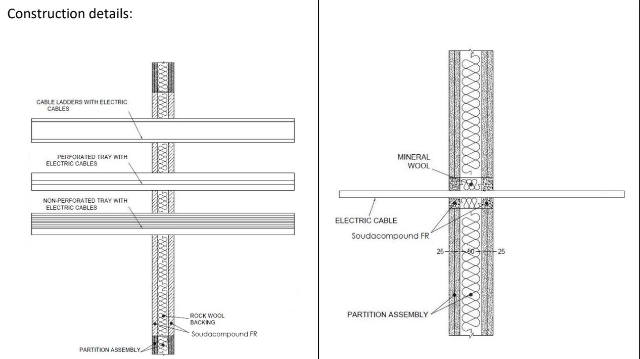
**A.5.1.1 Double side penetration seal with cables**
